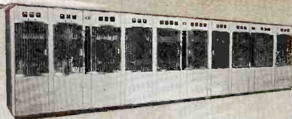
20 kw, for VHF Type TT-20BL/H (All Air-Cooled)
